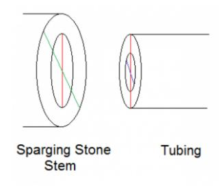
In another type of sparging stone, the OD of the sparging stone stem and the ID of the low pressure tubing are the same (**blue** lines). The ID of the sparging stone stem (**orange**) is smaller than the OD of the low pressure tubing (**red**).
